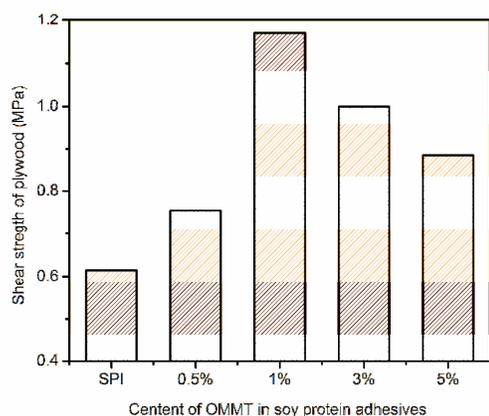
Figure 3: Shear strength of poplar plywood bonded with soy protein adhesive in the absence and presence of OMMT
