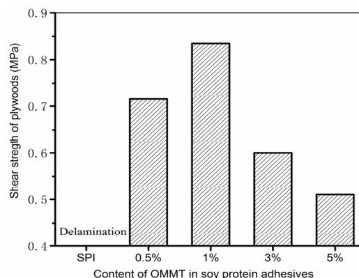
Figure 4: Shear strength of poplar plywood bonded with soy protein adhesive in the absence and presence of OMMT after water soaking tests
