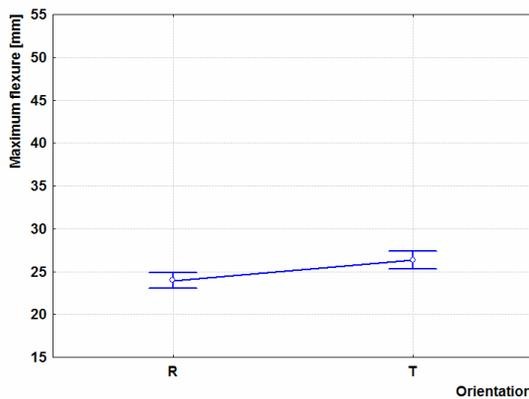
Figure 5: Influence of orientation on maximum flexure (95% confidence intervals)
