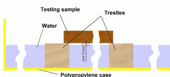
Figure 2: Schematic demonstration of testing sample positioned during plasticizing by microwave heating
