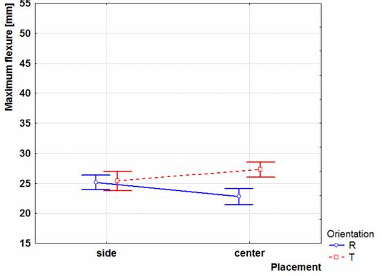
Figure 10: Influence of placement and orientation on maximum flexure (95% confidence intervals)
