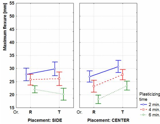
Figure 15: Influence of orientation, placement and plasticizing time on maximum flexure (95% confidence intervals)
