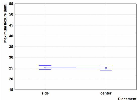
Figure 6: Influence of placement on maximum flexure (95% confidence intervals)
