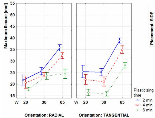
Figure 18: Influence of plasticizing time, orientation, moisture content, and placement at side on maximum flexure (95% confidence intervals)
