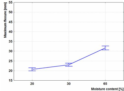
Figure 4: Influence of moisture content on maximum flexure (95% confidence intervals)
