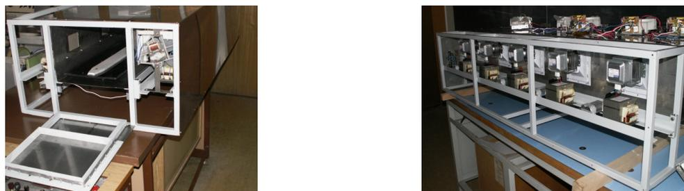
Figure 1: Microwave plasticizing device: a) overview; b) placement of magnetrons
