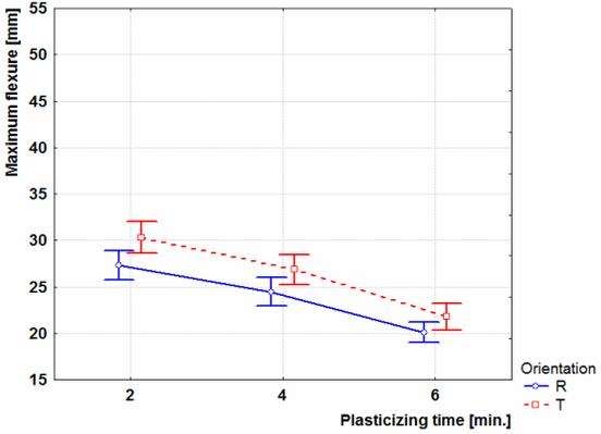
Figure 8: Influence of plasticizing time and orientation on maximum flexure (95% confidence intervals)
