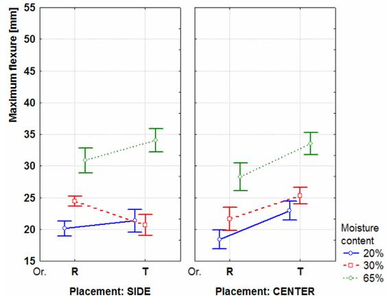
Figure 16: Influence of placement, moisture content and orientation on maximum flexure (95% confidence intervals)
