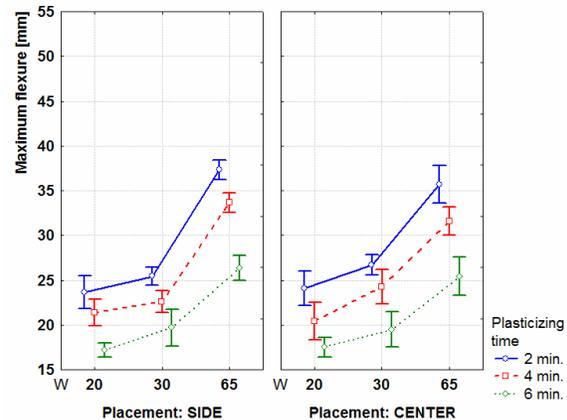
Figure 14: Influence of placement, plasticizing time and moisture content on maximum flexure (95% confidence intervals)
