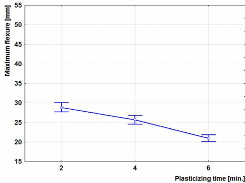
Figure 3: Influence of plasticizing time on maximum flexure (95% confidence intervals)
