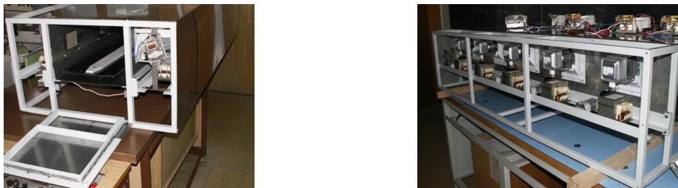
Figure 1: Microwave plasticizing device: a) overview; b) placement of magnetrons
