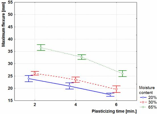
Figure 7: Influence of plasticizing time and moisture content on maximum flexure (95% confidence intervals)
