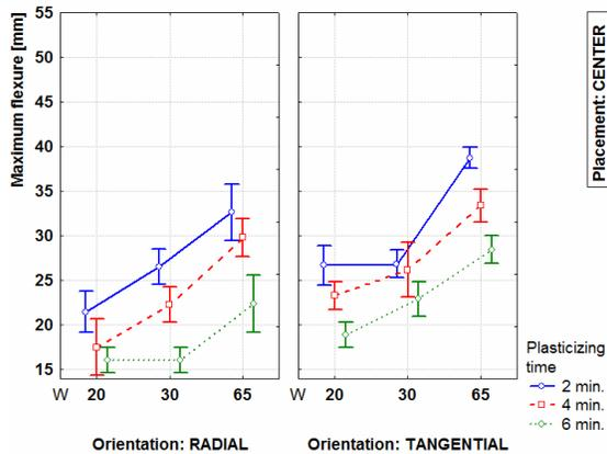
Figure 17: Influence of orientation, moisture content, plasticizing time and placement at center on maximum flexure (95% confidence intervals)
