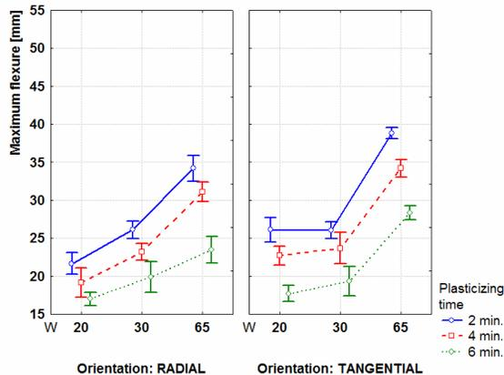
Figure 13: Influence of orientation, plasticizing time and moisture content on maximum flexure (95% confidence intervals)
