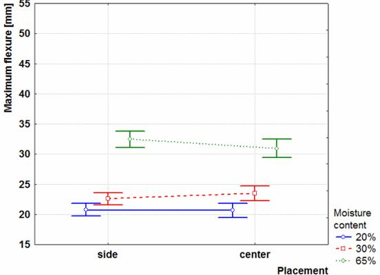
Figure 9: Influence of placement and moisture content on maximum flexure (95% confidence intervals)
