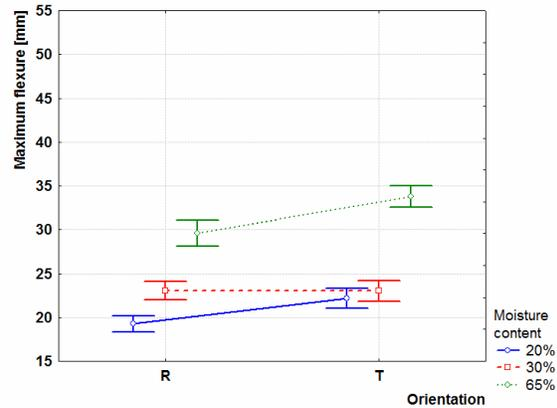
Figure 12: Influence of orientation and moisture content on maximum flexure (95% confidence intervals)
