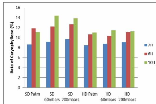
Figure 5: Evolution of caryophyllene yield (%) versus extraction time by different methods: steam distillation (SD) and hydrodistillation (HD) at atmospheric pressure, 60 mbars and 200 mbars
