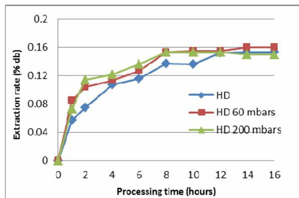
Figure 3: Extraction kinetics of maritime pine wood waste by hydrodistillation (HD) at atmospheric pressure, 60 mbars and 200 mbars
