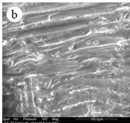
Figure 8: Maritime pine wood after 10 hours of steam distillation under vacuum (a) and hydrodistillation under vacuum (b) at 60 mbars (400x)
