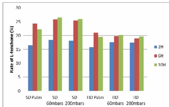
Figure 4: Evolution of L-fenchone yield (%) versus extraction time by different methods: steam distillation (SD) and hydrodistillation (HD) at atmospheric pressure, 60 mbars and 200 mbars
