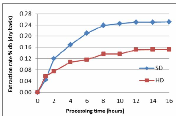
Figure 1: Extraction kinetics of maritime pine wood waste by steam distillation (SD) and hydrodistillation (HD)
