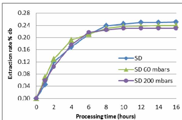
Figure 2: Extraction kinetics of maritime pine wood waste by steam distillation (SD) at atmospheric pressure, 60 mbars and 200 mbars
