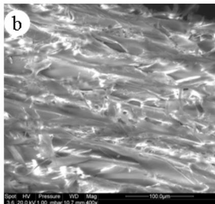
Figure 7: Maritime pine wood after 10 hours of steam distillation (a) and hydrodistillation (b) at normal pressure and temperature (400x)
