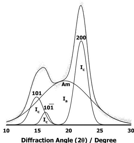
Figure 1: X-ray diffractogram of soda-AQ pulp showing fitted crystalline regions and the amorphous halo
