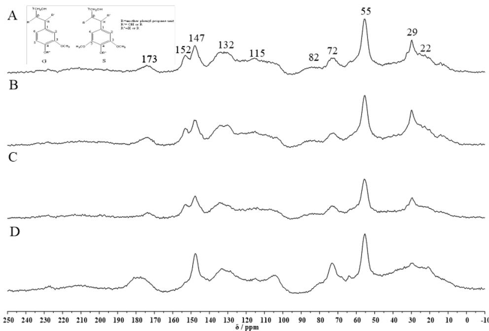
Figure 4: CP/MAS  $^{13}C$  solid-state NMR of lignins obtained from (A) OSP1, (B) OSP2, (C) OSP3 and (D) SAQP
