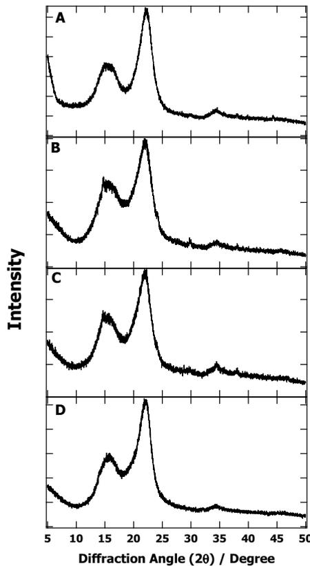
Figure 2: X-ray diffractogram of BP obtained from (A) OSP1, (B) OSP2, (C) OSP3, and (D) SAQP
