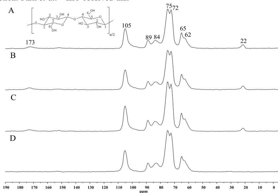
Figure 3: CP/MAS  $^{13}C$  solid-state NMR of BPs obtained from (A) OSP1, (B) OSP2, (C) OSP3 and (D) SAQP
