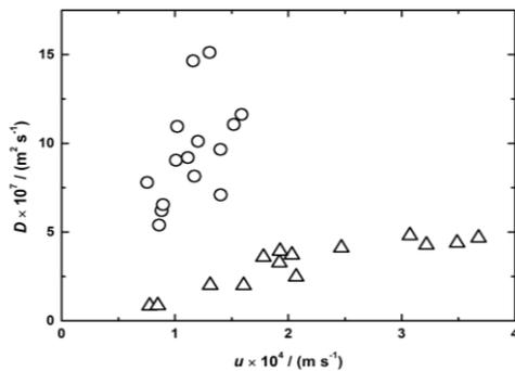
Figure 5: Influence of superficial wash liquid velocity on axial dispersion coefficient for spruce (O) and hardwood (Δ) (ref.<sup>25</sup>) pulps
