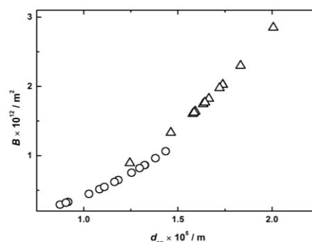
Figure 10: Bed permeability as a function of equivalent pore diameter for spruce (○) and hardwood (△) pulps
