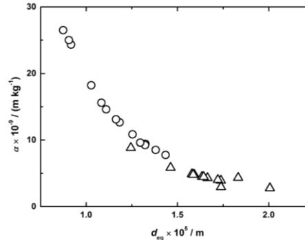
Figure 8: Specific bed resistance as a function of equivalent pore diameter for spruce (O) and hardwood (Δ) pulps
