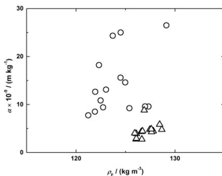
Figure 7: Specific bed resistance as a function of bed consistency for spruce (O) and hardwood (Δ) pulps
