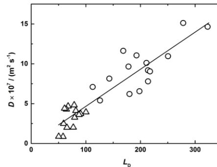
Figure 6: Influence of normalised dispersion length on axial dispersion coefficient for spruce (O) and hardwood (Δ) pulps (solid line Eq. (11))
