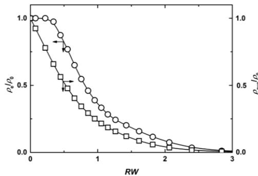
Figure 2: Typical breakthrough curve,  $\rho_e/\rho_0$  vs.  $RW$  ( $\circ$ ), and normalised average alkali lignin concentration in the pulp bed,  $\rho_{avg}/\rho_0$  ( $\square$ ), for displacement washing of kraft spruce pulp
