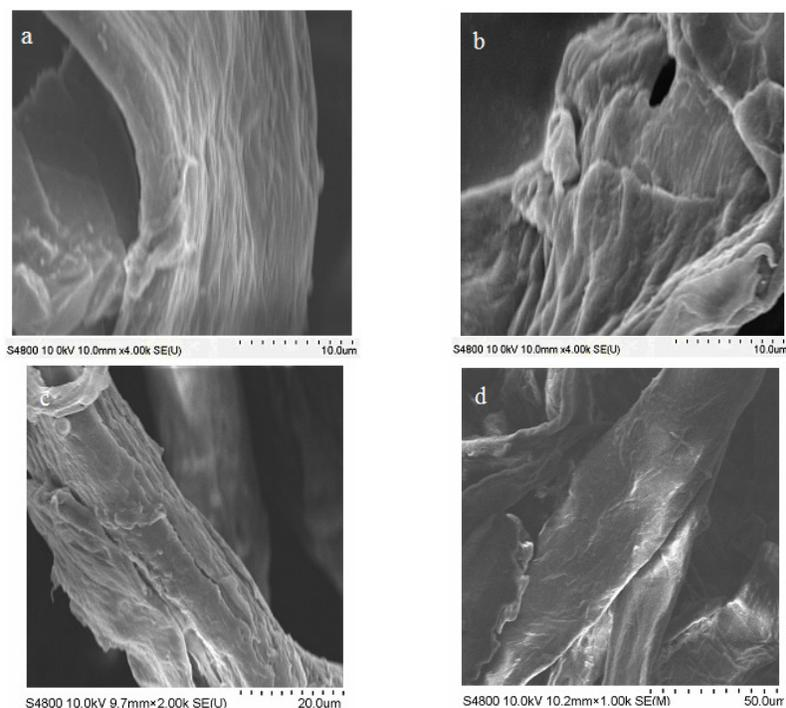
Figure 2: SEM images of raw cellulose (a), thiol-functionalized cellulose (TFC) (b), TFC after adsorption (c), and TFC after desorption (d)
