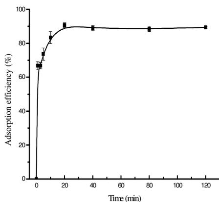
Figure 5: Adsorption efficiency *versus* adsorption time
