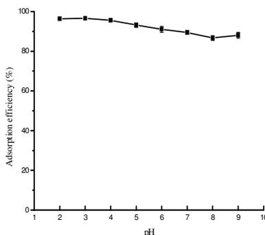
Figure 4: Effect of pH on Hg(II) adsorption by TFC
