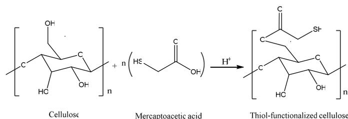
Figure 1: Schematic reaction of cellulose and mercaptoacetic acid
