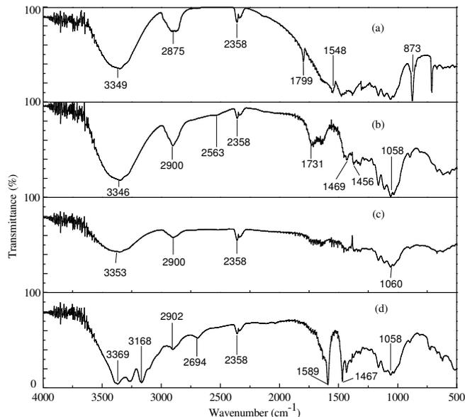
Figure 3: FTIR spectra of raw cellulose (a), thiol-functionalized cellulose (TFC) (b), TFC after adsorption (c), and TFC after desorption (d)
