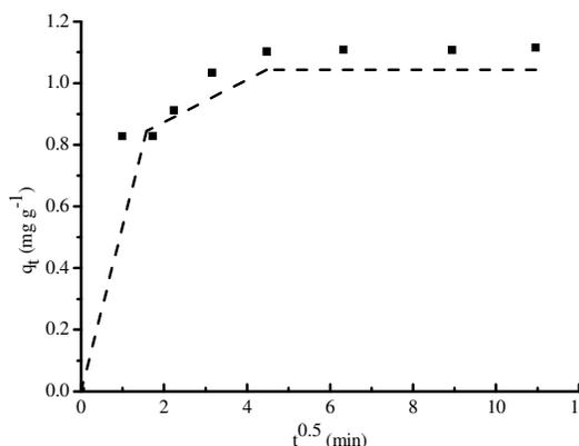
Figure 6: Fitting curve of Weber-Morris model for the adsorption of Hg(II) by TFC
