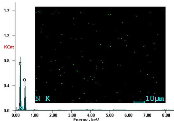
Figure 3: EDAX analysis of PU+EM blend film
