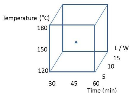
Figure 1: 2<sup>3</sup> Factorial design with time, temperature and liquid/solid ratio as variables
