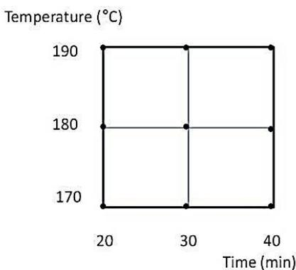
Figure 2: Central Composite Face-Centered Design with time and temperature as variables
