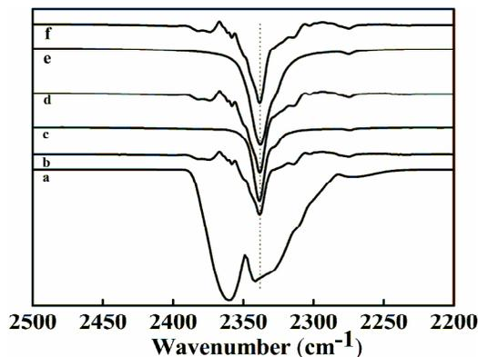
Figure 4: Comparison of FTIR spectra for the antisymmetric stretching mode of CO<sub>2</sub> for (a) scCO<sub>2</sub>; scCO<sub>2</sub> containing ethyl acetate; (b) 2 wt%; (c) 3 wt%; (d) 4 wt%; (f) 5 wt%
