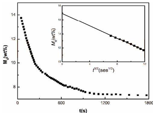
Figure 1: Desorption curve of scCO<sub>2</sub> in cellulose nitrate (Inset plot of  $M_d$  as a function of  $t^{1/2}$  for an initially short desorption time)
