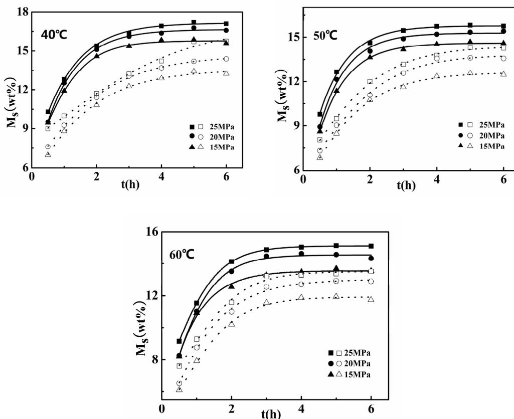
Figure 5: Solubility curves at different saturation pressures (15 MPa, 20 MPa, 25 MPa) and temperatures (40 °C, 50 °C, 60 °C) (Dotted line: scCO<sub>2</sub>; solid line: scCO<sub>2</sub> containing ethyl acetate)
