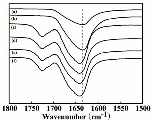
Figure 3: FTIR spectra of the nitrate ester group of cellulose nitrate for: (a) before; and immediately after scCO<sub>2</sub> treatment containing ethyl acetate (b) none; (c) 2 wt%; (d) 3 wt%; (e) 4 wt%; (f) 5 wt%
