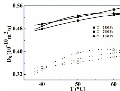
Figure 9: Influence of saturation pressure and temperature on the sorption diffusivity (Dotted line: SC-CO<sub>2</sub>; solid line: SC-CO<sub>2</sub> containing ethyl acetate)
