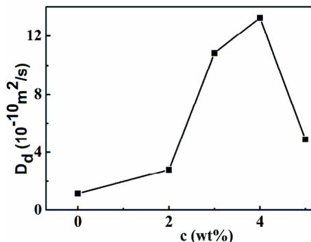
Figure 11: Plot of desorption diffusivity against ethyl acetate content
