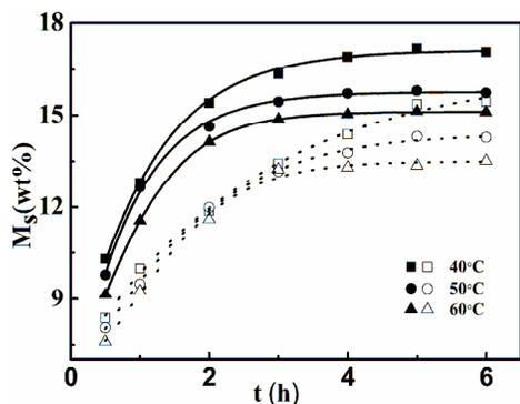
Figure 6: Solubility curves at different saturation temperatures under 25 MPa (Dotted line: scCO<sub>2</sub>; solid line: scCO<sub>2</sub> containing ethyl acetate)
