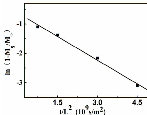
Figure 7: Plot of  $\ln(1-M_s/M_\infty)$  against  $(t_s / L^2)$  after different saturation time
