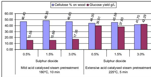
Figure 3: Glucose yield under different pretreatment conditions
