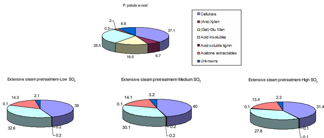
Figure 1: Yield balance of wood component after extensive acid catalysed steam pretreatment of *Pinus patula* wood
