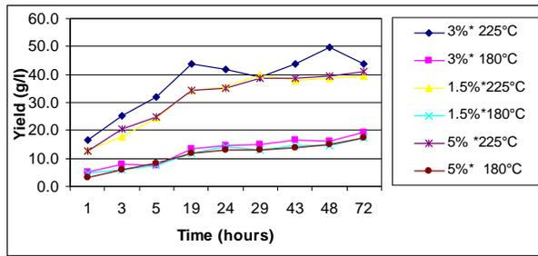
Figure 2: Glucose yield from hydrolysis of *P. patula* wood waste (\* sulphur dioxide)
