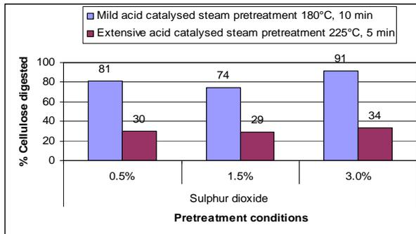
Figure 4: Percentage of cellulose digested in enzymatic hydrolysis
