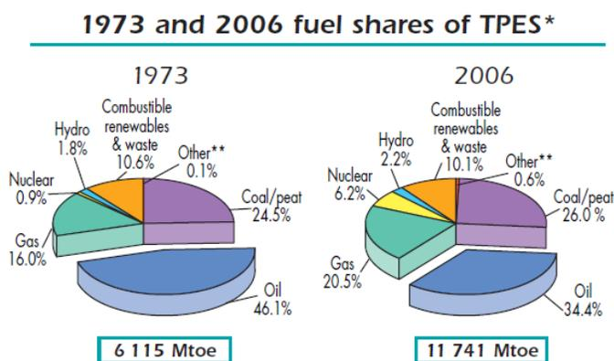
Figure 1: Evolution<sup>1</sup> (1971-2006) of world total primary energy supply (TPES)\* by fuel (Mtoe)
