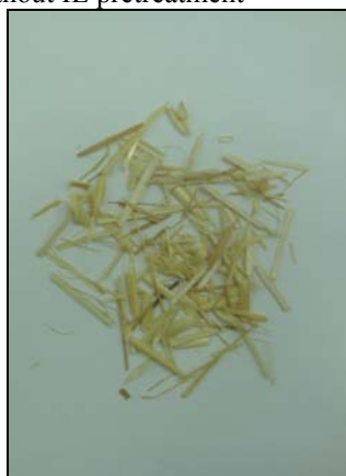
Figure 3: Wheat residues a) without pretreatment, b) with pretreatment (150 °C for 60 min)
