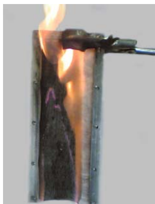
Figure 1: Mostashari's Flammability Tester shortly before the end of the experiment with a low addition of red phosphorus
