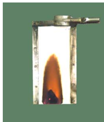
Figure 2: Mostashari's Flammability Tester during the test with a low addition of sodium polymetaphosphate
