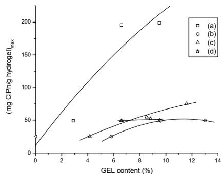
Figure 10: Variation of the maximum drug amount included as a function of the gelatin (GEL) content for different crosslinking reaction parameters: a – gelatin content in the polymer mixture; b – polymer mixture/crosslinking agent ratio; c – reaction duration; d – total polymer concentration in solution
