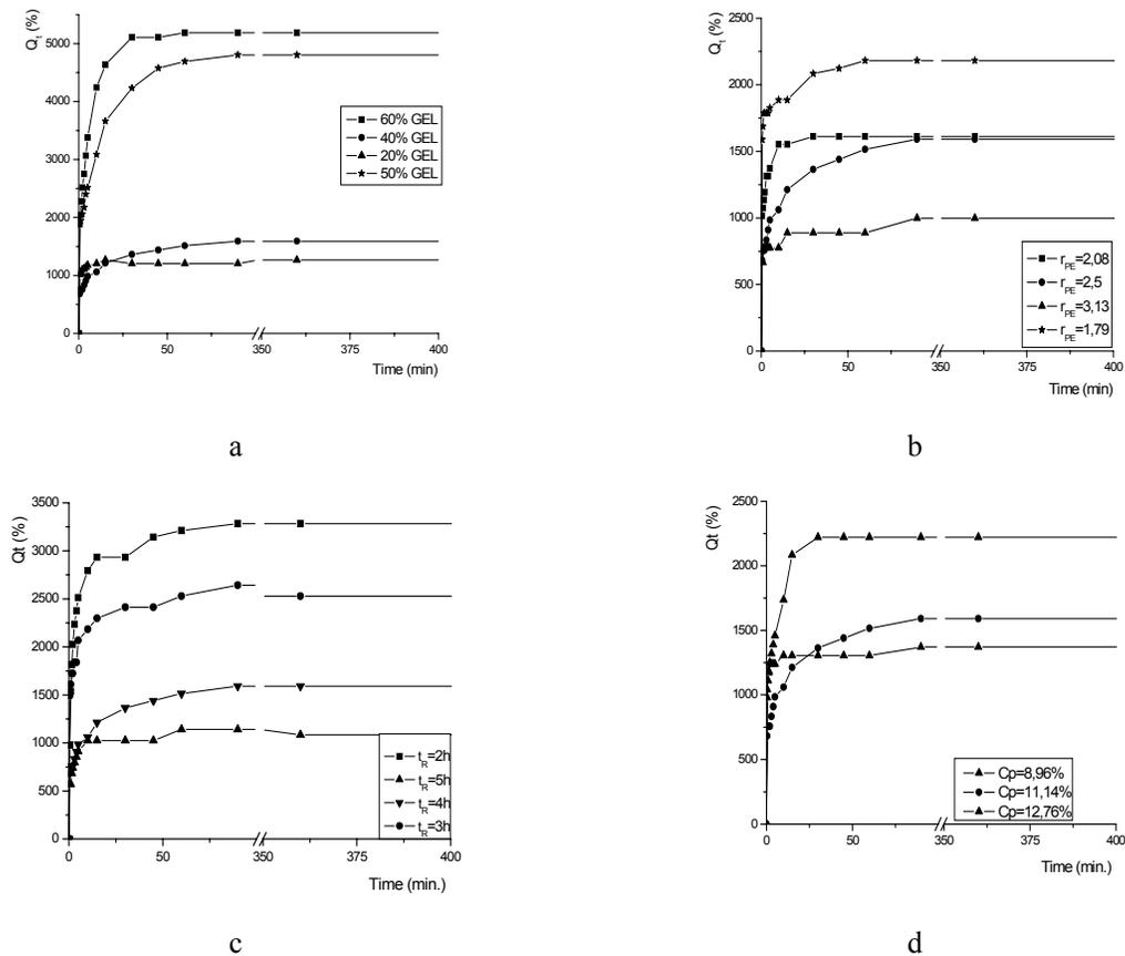
Figure 8: Variation of maximum swelling ratio as a function of the gelatine (GEL) content for different crosslinking reaction parameters: a – gelatin content in the polymer mixture; b – polymer mixture/crosslinking agent ratio; c – reaction duration; d – total polymer concentration in the solution
