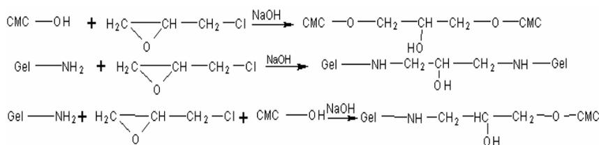
Figure 1: Crosslinking reactions with epichlorohydrin, occurring in carboxymethylcellulose-gelatin mixture
