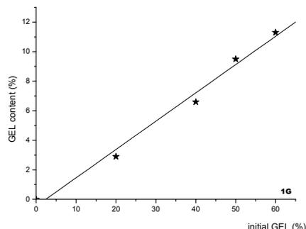
Figure 4: Gelatin (GEL) composition of hydrogels as a function of the initial gelatine (GEL) concentration in the polymer mixture (crosslinking conditions:  $T = 45\text{ }^{\circ}\text{C}$ ;  $t_R = 4\text{ h}$ ;  $r_{PE} = 2.5$ ;  $C_p = 11.135\%$ )
