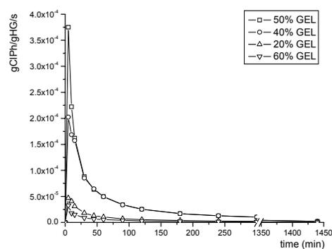
Figure 12: Chloramphenicol (CIPh) release kinetics of hydrogels differing as to the gelatin (GEL) composition of the initial polymer mixtures
