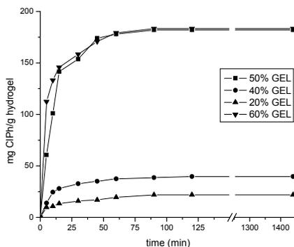
Figure 11: Chloramphenicol (CIPh) release kinetics of hydrogels differing as to the gelatin (GEL) content in the polymer mixture
