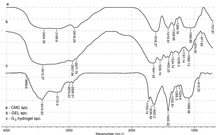
Figure 2: FTIR spectra for gelatine (GEL), carboxymethylcellulose (CMC) and gelatin-carboxymethylcellulose based hydrogel (CMC:GEL = 60:40, r<sub>PE</sub> = 2.5, t<sub>R</sub> = 4 h, C<sub>p</sub> = 11.135%, T = 45 °C)
