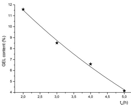
Figure 6: Variation of gelatin (GEL) content in hydrogels with crosslinking time (crosslinking conditions:  $T = 45\text{ }^{\circ}\text{C}$ ; CMC:GEL = 60:40;  $r_{PE} = 2.5$ ;  $C_p = 11.135\%$ )
