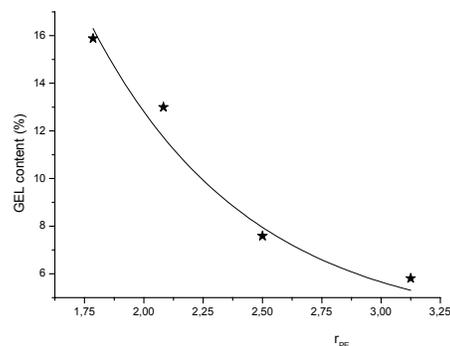
Figure 5: Influence of epichlorhydrin concentration on the gelatin (GEL) content of hydrogels (crosslinking conditions:  $T = 45\text{ }^{\circ}\text{C}$ ;  $t_R = 4\text{ h}$ ; CMC:GEL = 60:40;  $C_p = 11.135\%$ )
