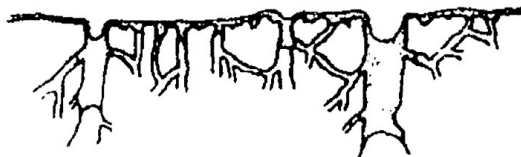
Figure 1: Capillary structure of paper 27,20
