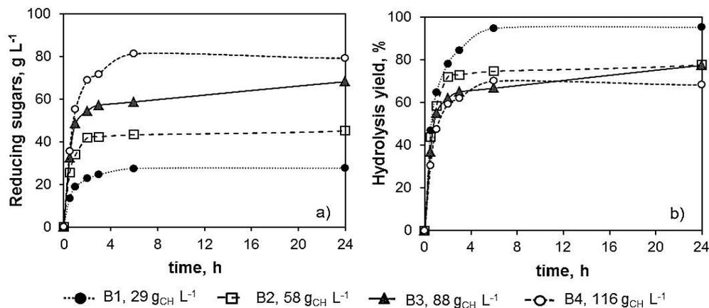
Figure 3: Enzymatic hydrolysis of unbleached pulp with Cellic<sup>®</sup> CTec2 (35 FPU  $\text{g}_{\text{CH}}^{-1}$ ), for different initial carbohydrate concentrations (29-116  $\text{g}_{\text{CH}} \text{L}^{-1}$ ), under batch conditions: a) reducing sugars produced, b) hydrolysis yield
