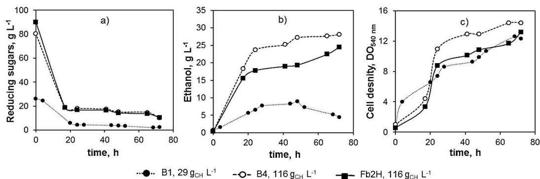
Figure 5: Ethanolic fermentation of enzymatic hydrolyzates of unbleached pulp (produced either in batch or in fed-batch enzymatic hydrolysis) with *Saccharomyces cerevisiae* ATCC 26602: a) reducing sugars consumption, b) ethanol production, c) cell density
