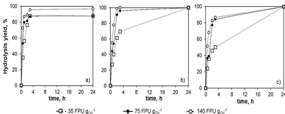
Figure 2: Enzymatic hydrolysis of unbleached pulp (equivalent to 25 g L<sup>-1</sup> of carbohydrates) with commercial cellulolytic enzymes: a) Cellic® CTec2 from Novozymes; b) Accellerase® 1500 from Genencor; and c) Dyadic® Cellulase CP from Dyadic
