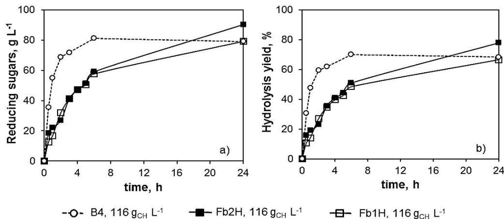
Figure 4: Enzymatic hydrolysis of unbleached pulp with Cellic® CTec2 (35 FPU g<sub>CH</sub><sup>-1</sup>, at the start-up of the reaction) under batch (B4) and fed-batch (Fb) conditions with a carbohydrate concentration equivalent to 116 g L<sup>-1</sup>: a) reducing sugars produced, b) hydrolysis yield
