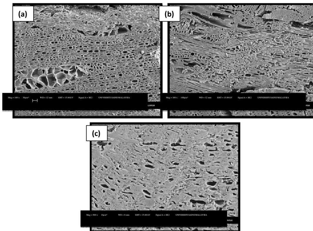
Figure 3: SEM micrographs showing cross section view of (a) NRS, native rice starch (b) EMRS, epichlorohydrin-modified rice starch and (c) EMRSUF, epichlorohydrin-modified rice starch with added urea formaldehyde resin panels with  $0.80 \text{ g/cm}^3$  target density manufactured with 20 min pressing time
