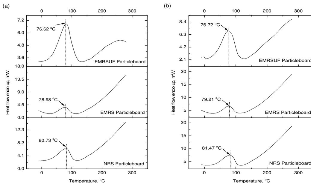
Figure 2: DSC curves of NRS, native rice starch; EMRS, epichlorohydrin-modified rice starch; and EMRSUF, epichlorohydrin-modified rice starch with added urea formaldehyde resin panels with 0.80 g/cm<sup>3</sup> target density manufactured with (a) 15 min, and (b) 20 min pressing time, respectively
