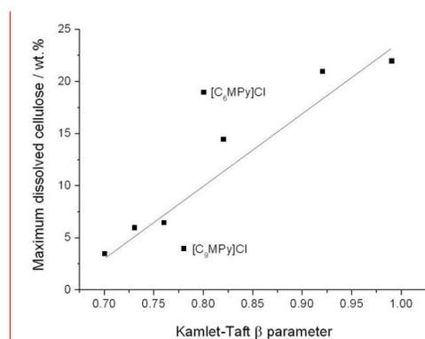
Figure 10: Correlation between the Kamlet-Taft  $\beta$  parameter values and the dissolving power of 1-alkyl-3-methylpyridinium-based ILs
