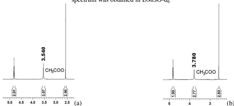
Figure 9: Partial <sup>1</sup>H-NMR spectrum for 1-butyl-3-methylpyridinium acetate (a), and solution of 1-butyl-3-methylpyridinium acetate with cellulose (b). <sup>1</sup>H-NMR spectra were obtained in CDCl<sub>3</sub>
