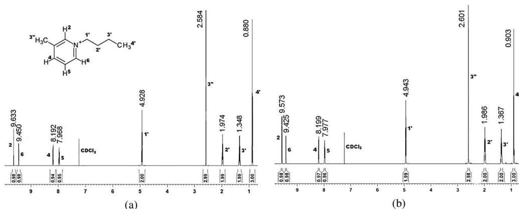
Figure 7: <sup>1</sup>H-NMR spectra for 1-butyl-3-methylpyridinium chloride (a), and solution of 1-butyl-3-methylpyridinium chloride with cellulose (b). <sup>1</sup>H-NMR spectra were obtained in CDCl<sub>3</sub>
