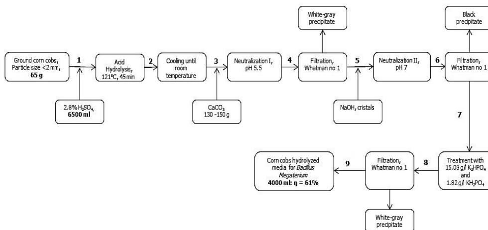
Diagram 1: Production and pretreatment of corn cob hydrolyzates
