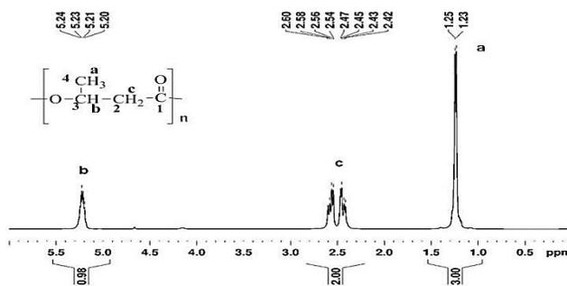
Figure 7:  $^1\text{H}$  NMR spectrum in  $\text{CDCl}_3$  corresponding to PHB
