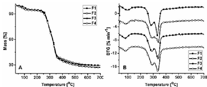
Figure 1: TG (A) and DTG (B) analysis of the fractions
