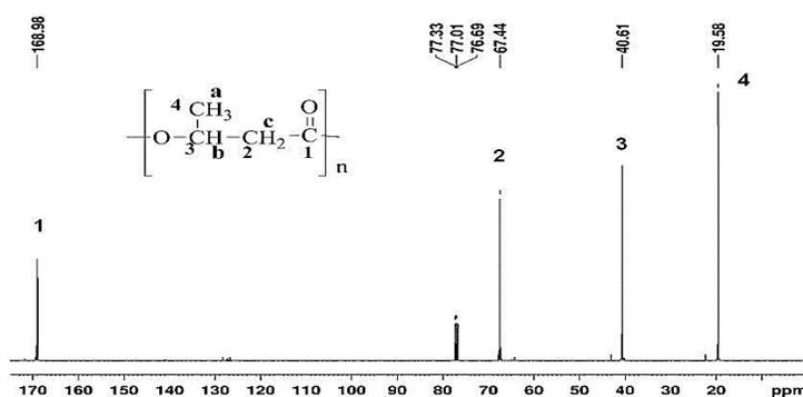
Figure 8:  $^{13}\text{C}$  NMR spectrum in  $\text{CDCl}_3$  corresponding to PHB
