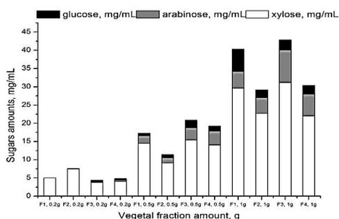
Figure 2: HPLC analysis of sugars in hydrolyzates obtained by method I
