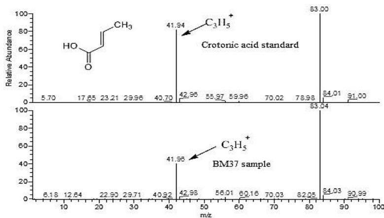
Figure 6: HPLC-MS spectrum of crotonic acid synthesized by *Bacillus* spp. BM 37 strain
