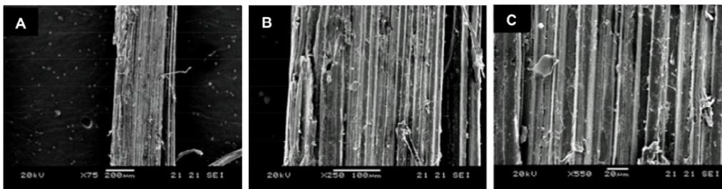
Figure 1: Cellular structures of sugarcane bagasse at (a) 75X, (b) 250X and (c) 550X – before chemical and biological treatments
