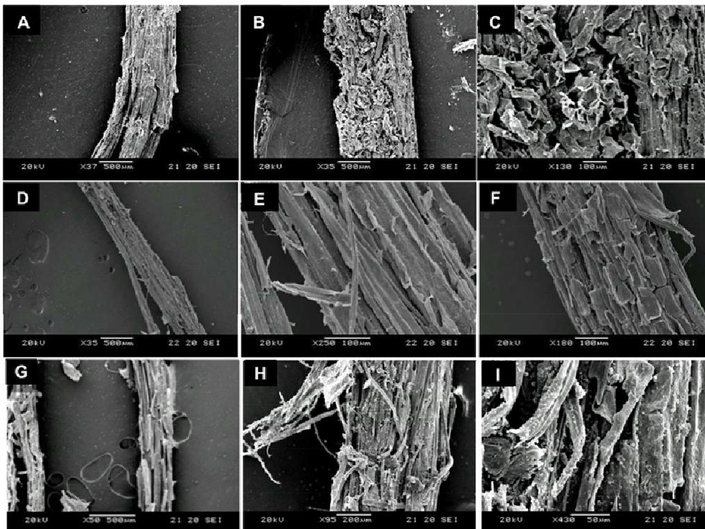
Figure 2: SEM images of chemically treated sugarcane bagasse: NaOH (A, B, C);  $\text{Ca}(\text{OH})_2$  (D, E, F) and NaOH +  $\text{Ca}(\text{OH})_2$  (G, H, I)
