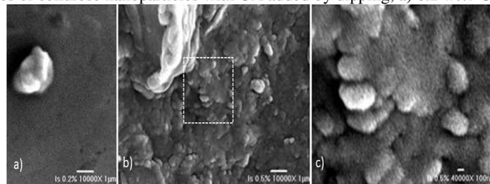
Figure 5: SEM analysis of cellulose nanoparticles with CA added *in situ*, a) 0.2 wt% CA, b) 0.5 wt% CA and c) zoom-in view of the square region
