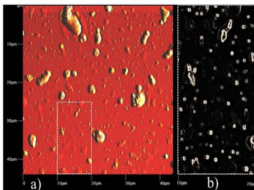
Figure 3: AFM images of pure cellulose nanoparticles on glass substrates; a) nanoparticles and aggregates; b) a magnified selected area
