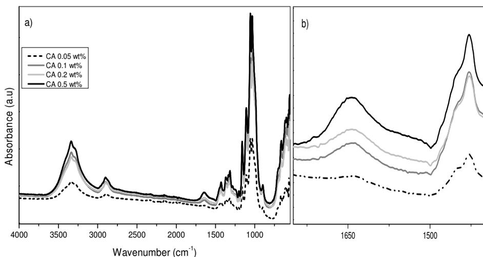
Figure 8: FTIR spectra of CA-containing cellulose nanoparticles obtained *in situ* at different CA concentrations, a) full view of the spectra b) zoom-in of the region between 1700-1400  $\text{cm}^{-1}$
