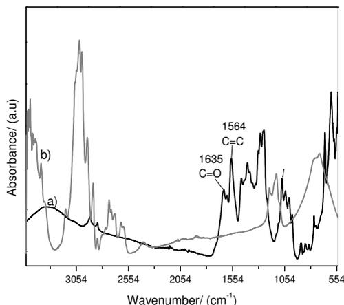
Figure 6: FTIR spectra of a) CA and b) pure cellulose nanoparticles
