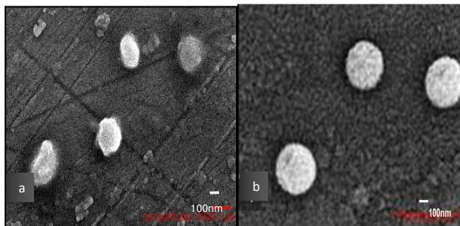
Figure 2: SEM images of pure cellulose nanoparticles on glass substrates a) at 10,000x and b) at 60,000x
