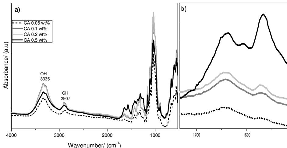
Figure 7: FTIR spectra of CA-containing cellulose nanoparticles obtained by dipping at different CA concentrations, a) full view of the spectra and b) zoom-in of the region between 1750-1400  $\text{cm}^{-1}$
