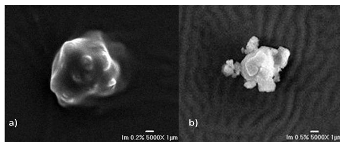
Figure 4: SEM images of cellulose nanoparticles with CA added by dipping, a) 0.2 wt% CA and b) 0.5 wt% CA
