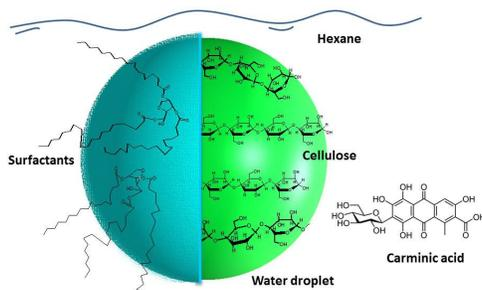
Figure 1: Schematic representation of cellulose chains in the hexane phase (inverse emulsion) and carminic acid
