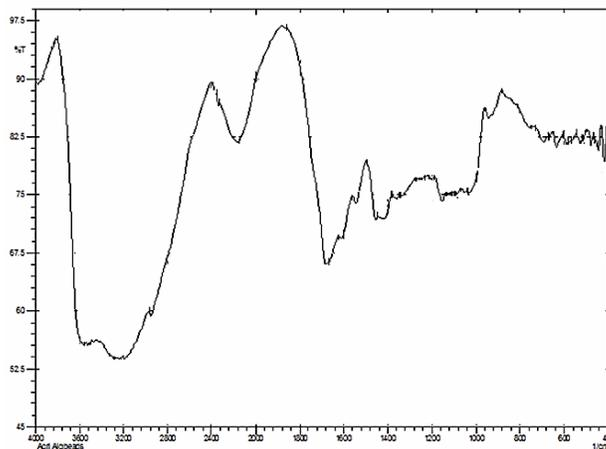
Figure 2: FTIR spectrum of CA/poly(AAm) composite beads
