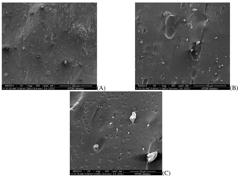
Figure 6: SEM images of CA/poly(AAm) composite beads with (A) 250X, (B) 1000X and (C) 4000X magnifications
