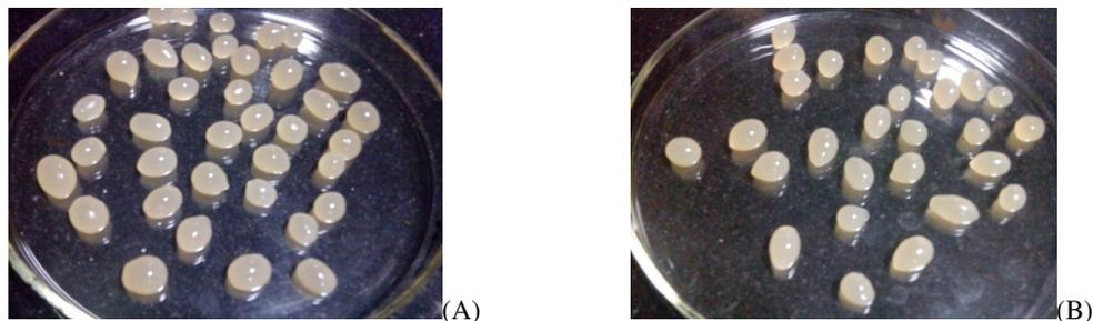
Figure 1: Optical image of (A) calcium alginate and (B) calcium alginate/poly(AAm) beads
