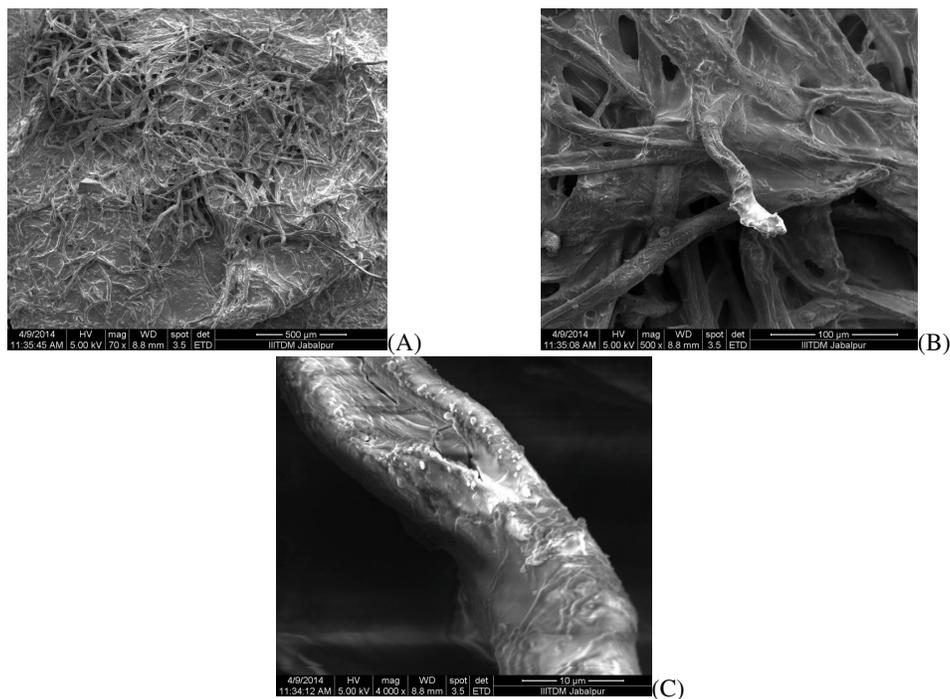
Figure 5: SEM images of CA beads at magnifications of (A) 70X, (B) 500X and (C) 4000X
