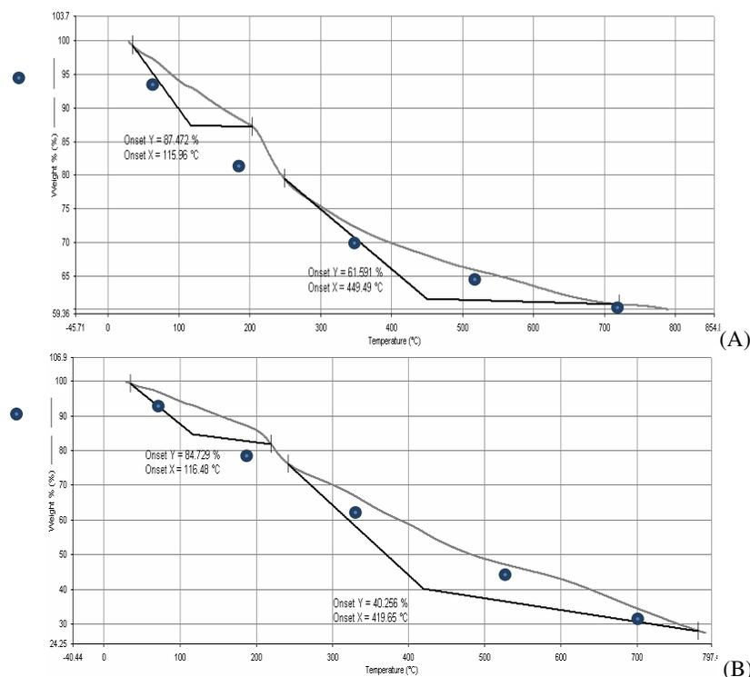
Figure 4: Thermograms of plain CA beads (A) and of CA/poly(AAm) beads (B)
