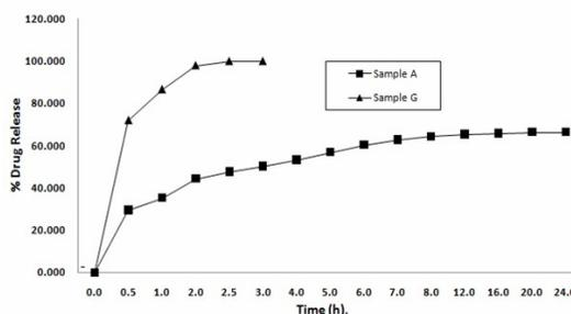
Figure 12: Release of model drug vitamin B<sub>2</sub> from the bead sample A (i.e. CA/poly(AAm) sample) and sample G (plain CA beads) in PF at 37 °C
