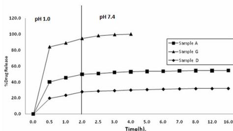
Figure 13: Drug release from plain CA bead sample G and samples A (CA/poly(AAm)) and D (CA/poly(AAm)) in media of varying pH (i.e. pH 1.0 for 2 h, followed by transfer to pH 7.4 for the rest of the period) at 37 °C
