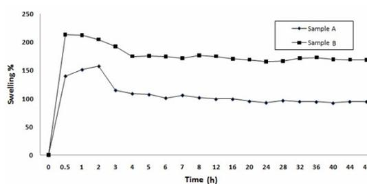
Figure 8: Percent swelling of CA/poly(AAm) bead samples A and B in physiological fluid of pH 7.4 at 37 °C
