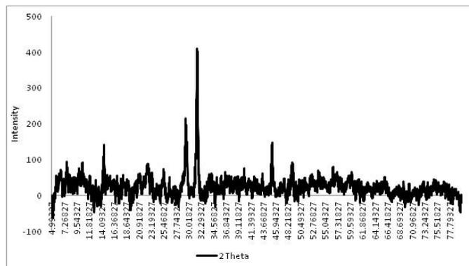
Figure 3: X-ray diffractogram of CA/poly(AAm) beads
