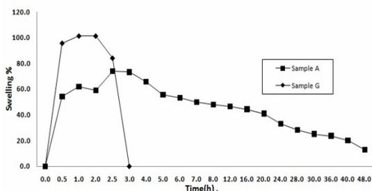
Figure 11: Stability of plain CA sample G and CA/poly(AAm) sample A beads in media of varying pH (i.e. pH 1.0 for 2 h, then transferred to pH 7.4 for the rest of the period) at 37 °C
