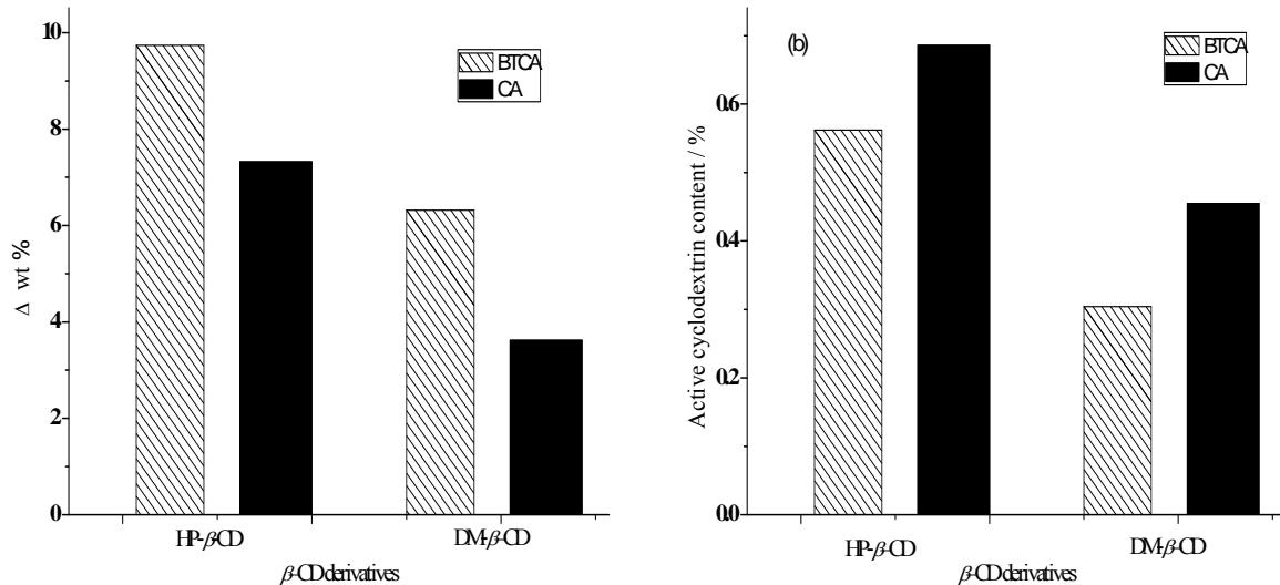
Figure 7: Cellulose beads grafting with HP- $\beta$ -CD and DM- $\beta$ -CD by different PCAs, in presence of PCAs (100 g  $\text{L}^{-1}$ ), at curing temperature of 180 °C for 5 min and with  $\text{NaH}_2\text{PO}_4/\text{CA}$  (30 g  $\text{L}^{-1}$ ) and  $\text{NaH}_2\text{PO}_4/\text{BTCA}$  (30 g  $\text{L}^{-1}$ ) as catalysts; (a) grafting rate; (b) active cyclodextrin content
