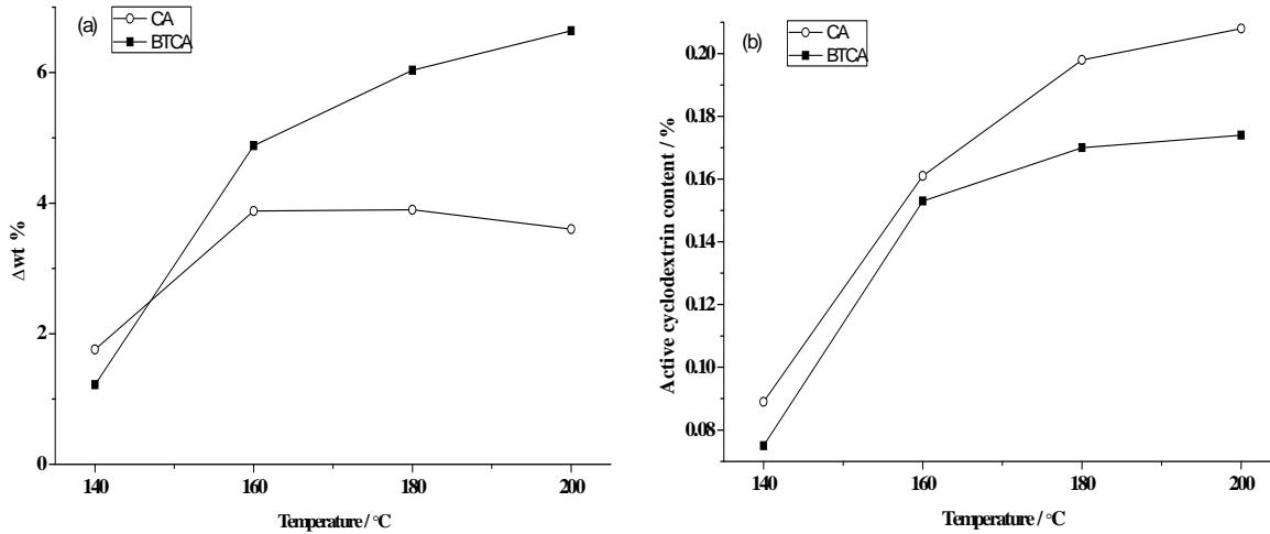
Figure 3: Influence of curing temperature (curing time = 5 min) on grafting, in presence of PCAs ( $100 \text{ g L}^{-1}$ ), with  $\text{NaH}_2\text{PO}_4$  ( $30 \text{ g L}^{-1}$ ) as catalyst and  $\beta$ -CD concentration of  $100 \text{ g L}^{-1}$ ; (a) grafting rate; (b) active cyclodextrin content
