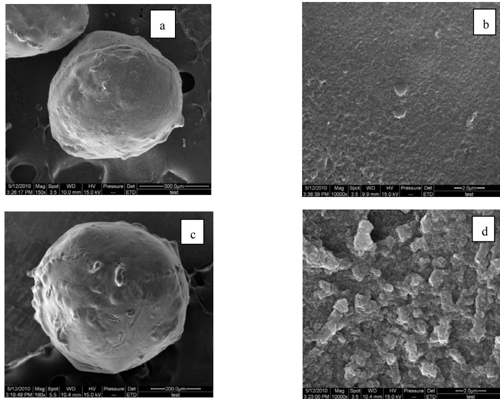
Figure 4: SEM pictures of cellulose beads (a, b) and  $\beta$ -CD grafted onto cellulose beads (c, d)
