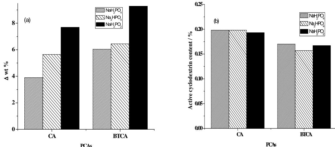
Figure 5: Influence of catalyst (30 g L<sup>-1</sup>) on grafting yield, in presence of PCAs (100 g L<sup>-1</sup>), at curing temperature of 180 °C for 5 min and with  $\beta$ -CD concentration of 100 g L<sup>-1</sup>;
