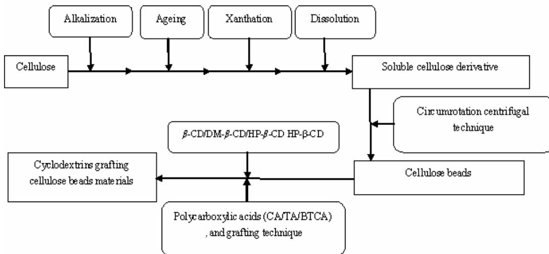
Scheme 1: Preparation procedure of cyclodextrins grafting onto cellulose bead material
