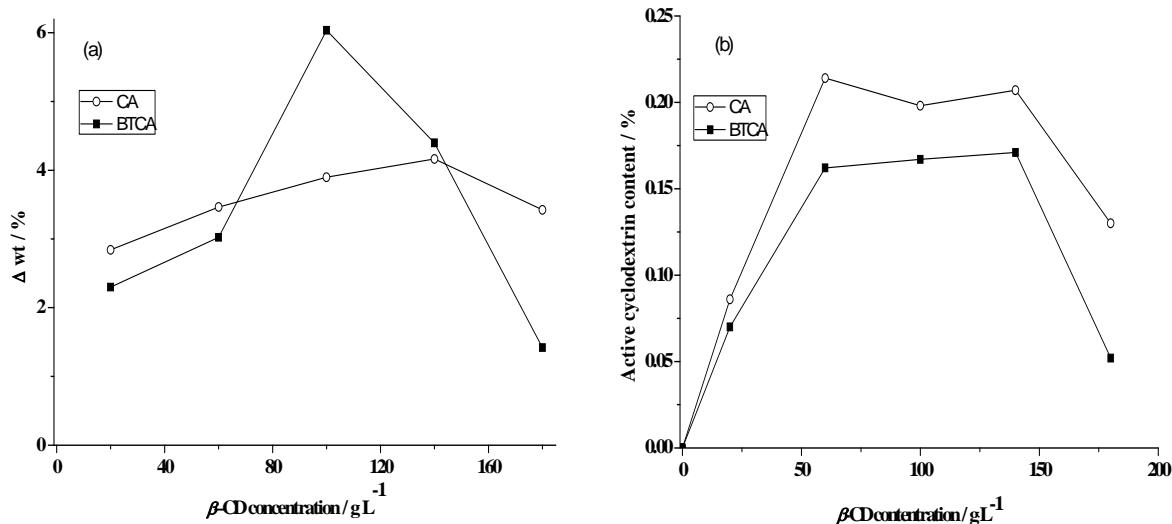
Figure 6: Influence of  $\beta$ -CD concentration in the impregnating bath on grafting yield, in presence of PCAs (100 g  $\text{L}^{-1}$ ), at curing temperature of 180 °C for 5 min and with  $\text{NaH}_2\text{PO}_4$  (30 g  $\text{L}^{-1}$ ) as catalyst; (a) grafting rate; (b) active cyclodextrin content
