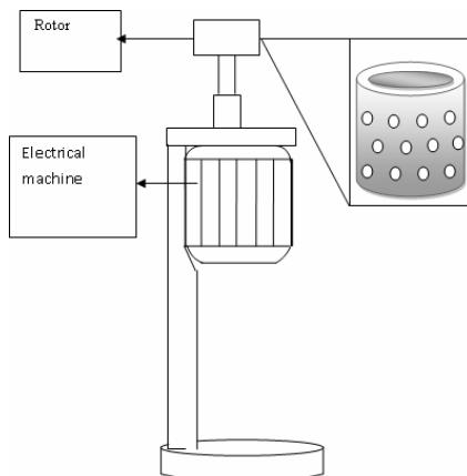
Scheme 3: Structure of centrifugal circumrotation machine
