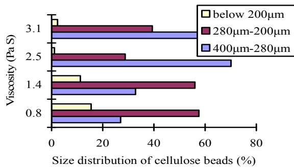
Figure 1: Viscosity of cellulose viscose vs. size distribution of cellulose beads
