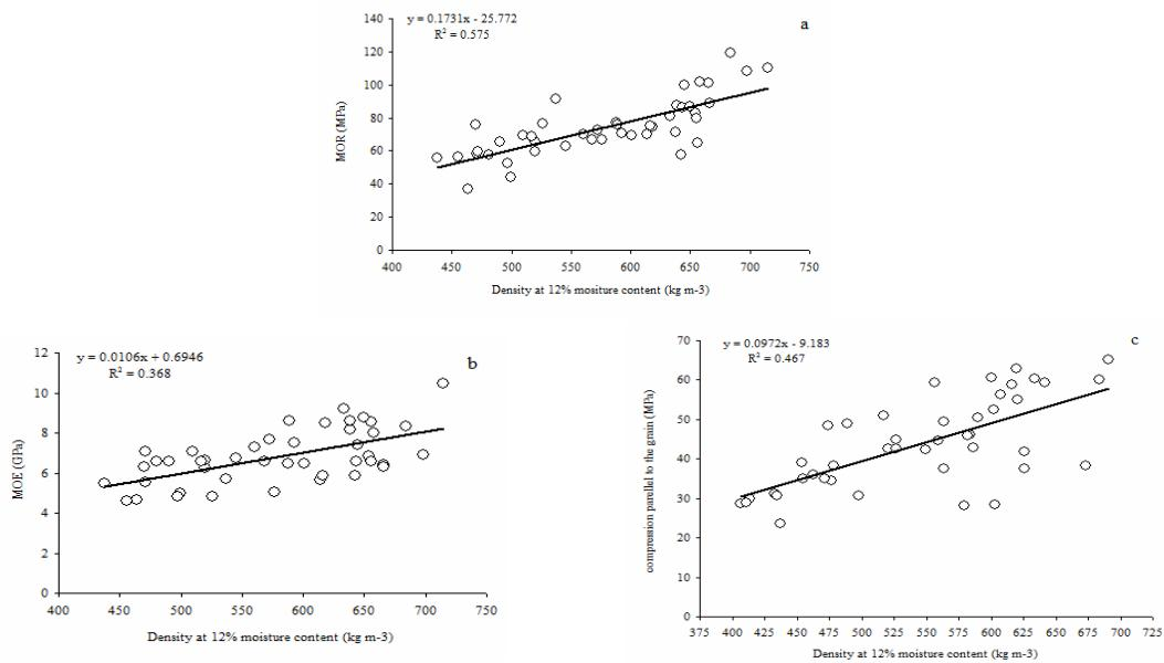
Figure 6: Relationship between density at 12% moisture content and modulus of rupture (a), modulus of elasticity (b), compression strength parallel to the grain (c) in eldar pine
