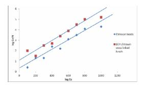
Figure 6: Linear model of Freundlich isotherm for Pb (II) adsorption onto chitosan beads and cross-linked chitosan beads
