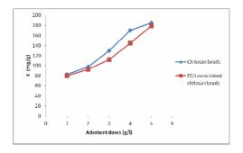
Figure 3: Effect of adsorbent dose on adsorption of Pb onto chitosan beads and ECH cross-linked chitosan
