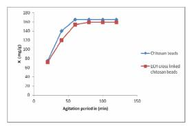
Figure 2: Effect of stirring time on adsorption of Pb onto chitosan beads and ECH cross-linked chitosan beads
