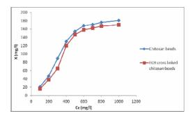
Figure 4: Adsorption isotherm of Pb onto chitosan beads and ECH cross-linked chitosan beads
