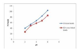
Figure 1: Effect of pH on Pb adsorption onto chitosan beads and cross-linked chitosan beads
