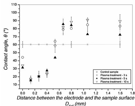
Figure 1: Contact angle variation ( $\theta$ , °) as a function of the distance between the electrode and the sample surface ( $D_{\text{SaE}}$ , mm) (the line represents the untreated control sample of wood (European beech (*Fagus sylvatica*)))
