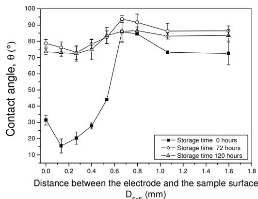
Figure 2: Effect of storage time after plasma treatment (0, 72 and 120 hours); plasma treatment time of 5 s, atmosphere – air
