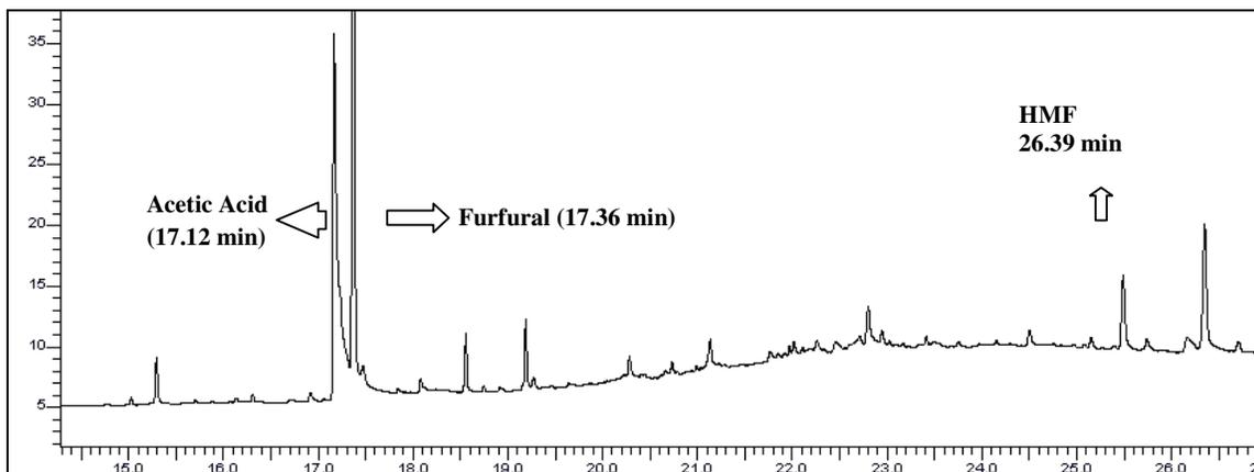
Figure 3: Gas chromatogram showing separation of acetic acid, furfural, HMF
