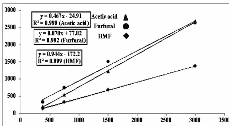
Figure 4: Calibration curves of major inhibitors based on response (ordinate) against concentration (abscissa)
